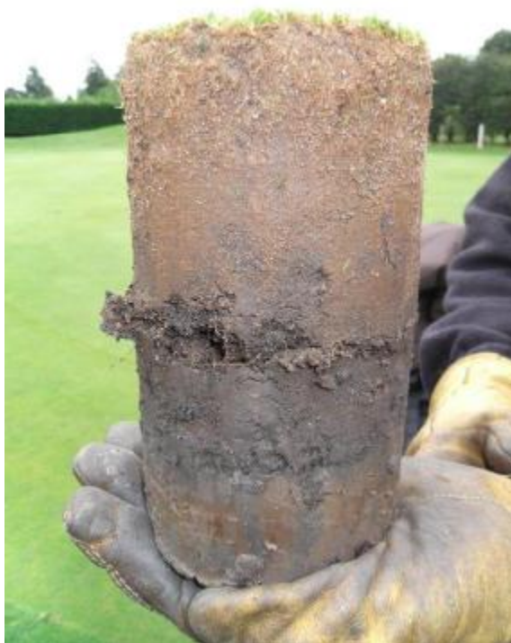
Photograph 2 soil profile taken from 4 th green showing heavy clay soil impeding drainage.
